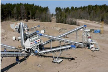
The OUTPUT is fine, sharply sorted crushed stone which can be the final product or used as an input material for the production of dry building materials
